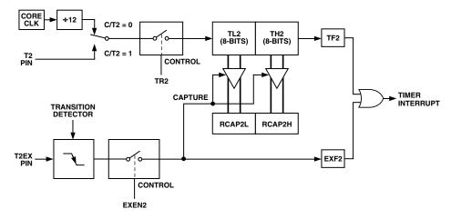
Figure 31. Timer/Counter 2, 16-Bit Capture Mode
